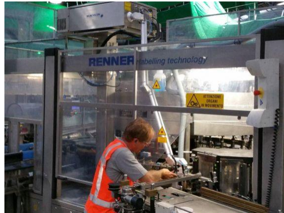
Service Engineer Eric Jobse installs a MundiScan laser
